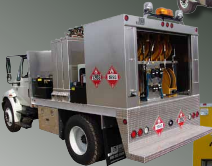
Oil products, water, and antifreeze tanks are safely stored in the enclosed body.
