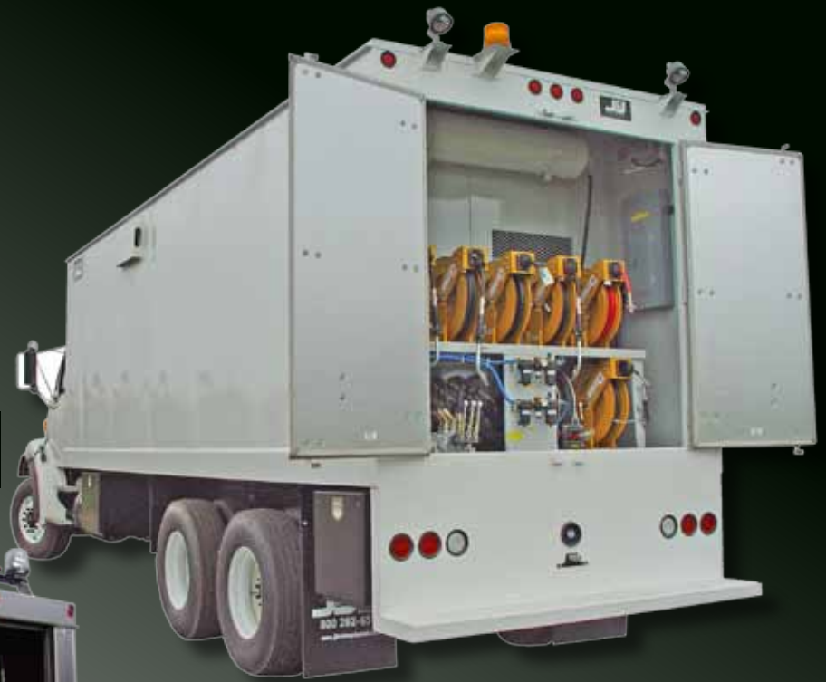
Oil products, water, and antifreeze tanks are safely stored in the enclosed body.
