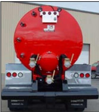
The truck can have either an extreme-duty rear bumper (shown in picture) or a heavy-duty rear bumper. The bumpers are built with a heavy structural 8" tubing and are coated with chip guard to provide extra grip when working on top. It features integrated tool boxes for storing fittings and chains for easy accessibility and a built-in step on the side for a user friendly step from ground level to top of bumper. The oil field tow flap is designed to pull 80,000 lbs.
