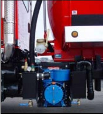
The truck features a plug and play pump package from Fruitland. This pump package has a stainless steel filter plumbed inline with both the vacuum and pressure side of the pump. It also contains a built-in secondary moisture trap and oil catch muffler that are all serviceable from ground level.
