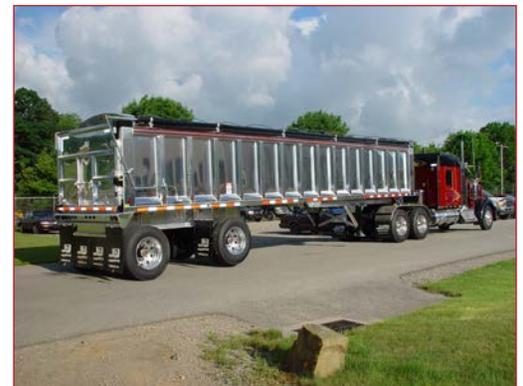
Convert from conventional gate to side swing gate in two quick steps with our easy-to-use combination tailgate.
