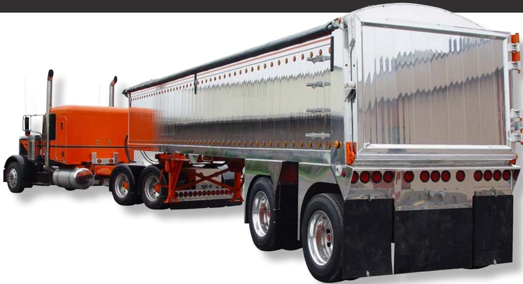
The EVO (smooth sides) series reinforced double wall side panels create a super strong side wall that is aerodynamic, insulated, and easy to clean.
