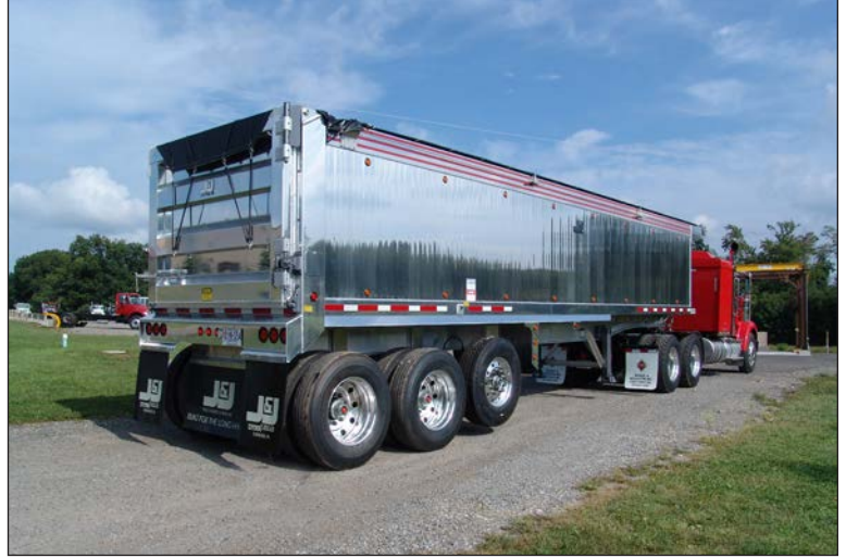
Mud guards, mud flaps, steps, and shovel hangers are standard on these trailers.
