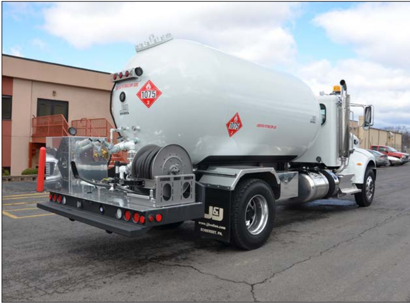
This photograph shows the optional spray-on protective coating that J&J offers. It outlasts and out-performs paints and undercoatings. It also prevents rust and corrosion and provides excellent impact and abrasion resistance.
