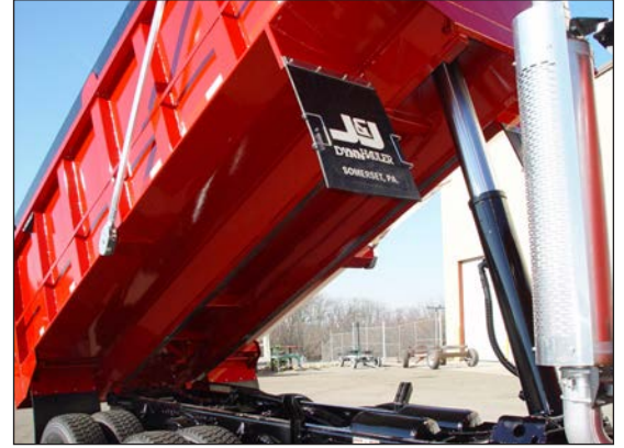
No crossmembers means lighter weight bodies.
