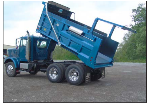
The air high lift tailgate option prevents tailgate damage from large objects and functions as a conventional tailgate for standard aggregate hauling.
