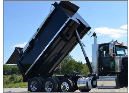
The absence of crossmembers reduces the weight of these trucks.
