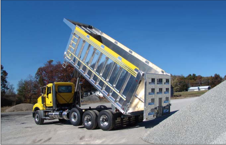
J&J Material Hauler dump bodies are designed to maximize payload.
