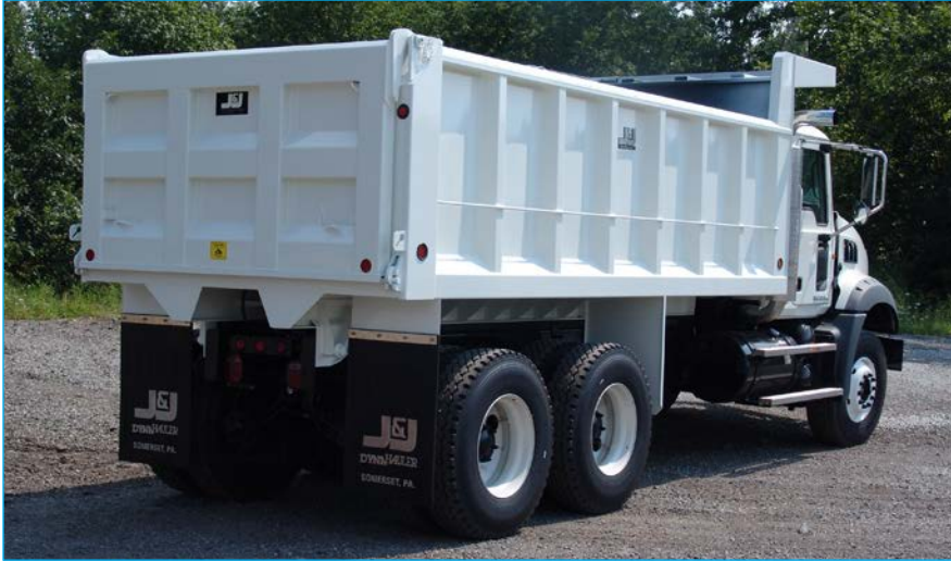
Sherwin-Williams Genesis® paint system provides a high gloss, extremely durable and resistant finish. All steel bodies are completely sandblasted for superior paint adhesion.
